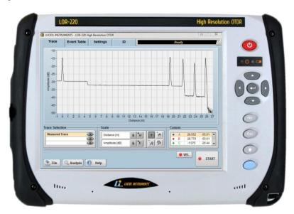
The LOR-220 from Luciol Instruments is a fully portable high resolution OTDR. It is similar in shape and feel to a standard OTDR, but achieves unprecedented resolution. The LOR-220 distinguishes events with 10 cm separation and has a 40 cm attenuation deadzone. Its unique dynamic range for short pulse lengths (over 12 dB for 1 ns pulses) enables to see through optical splitters, even over very short distances.
