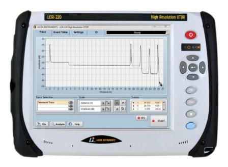
The LOR-220 from Luciol Instruments is a fully portable high resolution OTDR. It is similar in shape and feel to a standard OTDR, but achieves unprecedented resolution. The LOR-220 distinguishes events with 10 cm separation and has a 40 cm attenuation deadzone. Its unique dynamic range (> 12 dB for the 1 ns pulse-width) enables to see through optical splitters, even over very short distances.
