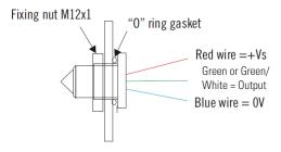
Note. LLPK1  $\,$  - Nitrile 'O' ring and Nickel plated brass M12 nut kit - is available as an optional extra.
