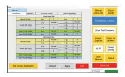
ConnectorView Plus software uses IEC 61300-3-35 as the default standard for its analysis, but the acceptance criteria can be modified to allow for different corporate standards.
