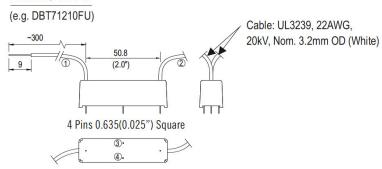
NOTE: PINS WHICH ARE NOT NUMBERED HAVE NO ELECTRICAL CONNECTION.
