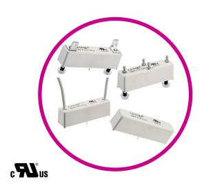
The DB(UL) series is a UL\* approved very high isolation voltages (up to 10kV) are achieved through the use of high vacuum reed switches with either rhodium or tungsten contacts and make these relays suitable for high reliability applications, such as cardiac defibrillators, test equipment and high voltage power supplies.
