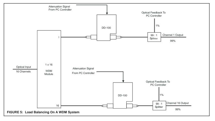
Multiplexed light from a trunk line is demultiplexed into individual signals as shown in Figure 5. They are of different intensities. The signals have to be balanced to avoid saturating any of the receivers. DD style attenuators are inserted between the WDM and the receiver modules. Whenever a receiver module is saturated, a signal is sent to the control computer to increase the attenuation to that module. Whenever the signal becomes too low, the control computer decreases the attenuation.
