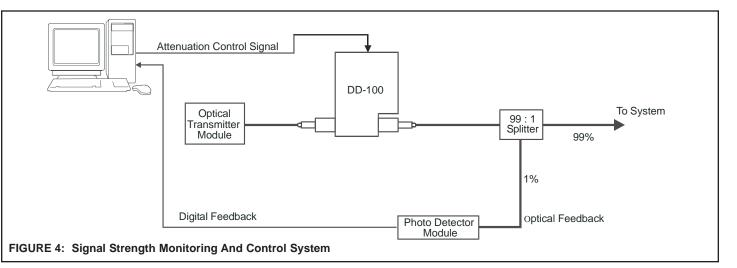
As illustrated in Figure 4 above, light from a transmission module is sent through a DD style attenuator before entering the transmission line. A 99:1 splitter is used to tap off a small monitor signal. This signal is measured with a photodiode module, which produces a digital representation of the light intensity. Based on this feedback, the computer adjusts the attenuator to set the output signal at the optimum intensity.
