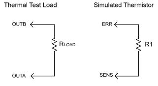
$R_{LOAD} = 1 \Omega$ . Rated >25 W R1 = 10 k $\Omega$ . <sup>1</sup>/<sub>4</sub> W resistor
