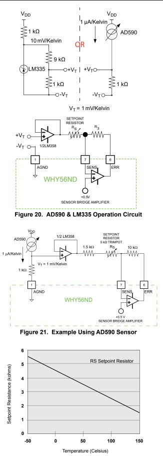
Figure 22. Example Setpoint Resistance vs. AD590 Temperature
