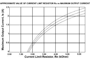
Figure 5. Resistor Value vs. Output Current
