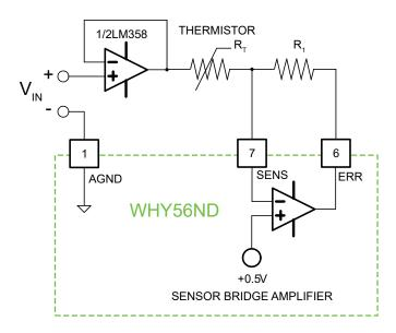
Figure 16. External Voltage Control Using Thermistor Sensors
