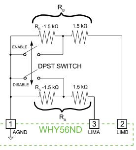
Figure 7. Enable/Disable Output Current Circuit
