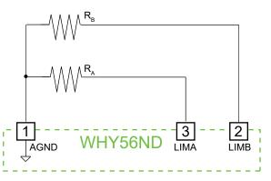
Figure 4. Fixed Heat and Cool Current Limits
