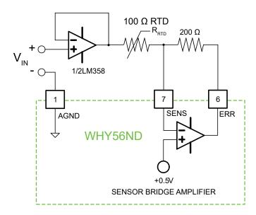
Figure 19. Example Using a 100  $\Omega$  RTD with External Voltage Control
