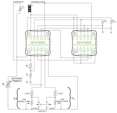
Figure 11. Boosting Output Current Drive
