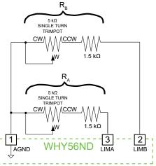
Figure 6. Independently Adjustable Heat and Cool Current Limits
