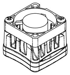
Figure 13. WHY56ND Assembled with Heatsink & Fan
