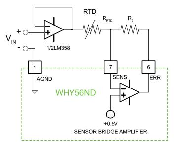
Figure 18. External Voltage Control Using RTD Sensors
