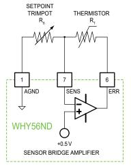
Figure 8. Thermistor Operation Circuit
