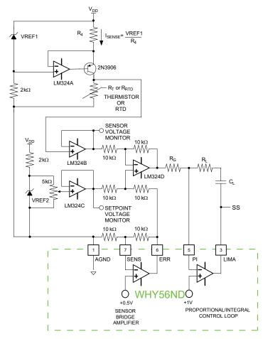
Figure 10. Monitor Setpoint and Actual Sensor Voltages Circuit
