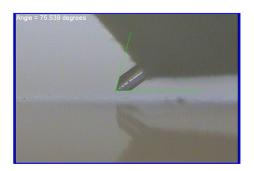
NOVA<sup>TM</sup>'s Profile Videoscope allows the real-time monitoring of component polishing. This videoscope aids with bare fiber/component positioning and confirms process completion. Teamed with measurement software, this system verifies the endface geometry of fibers, waveguides and arrays.
