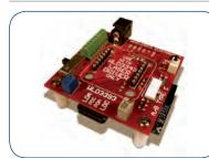
Use the Evaluation Boards to rapidly prototype a complete laser diode control system using the cutting edge technology of the Laser Diode Driver, Onboard switches, connectors,
