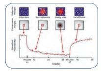
The technology uses а fluorescence microscope equipped with a dichroic mirror that couples a IR-Laser into the path of fluorescence light. The heating laser is focused with the same objective used for fluorescence detection.
