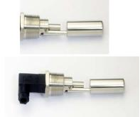
SSH66XE are externally mounted horizontal float switches with 3/4"NPT thread.. The float is of 316L Stainless Steel and the stem is of 304 Stainless Steel.
