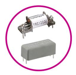
High current capability is achieved through the use of two reed switches in parallel. Open frame and covered construction are available, depending on voltage isolation requirements.
