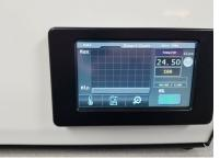
Thermocouple based P.I.D. temperature controller:
