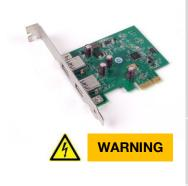
An external USB 3.0 host controller board comes along with the camera.
