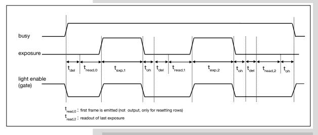
$\begin{array}{ll} t_{td}\text{:} & \text{trigger delay (incl. jitter)} \\ t_{\text{read}}\text{:} & \text{readout time} \\ t_{del}\text{:} & \text{delay time} \end{array}$
