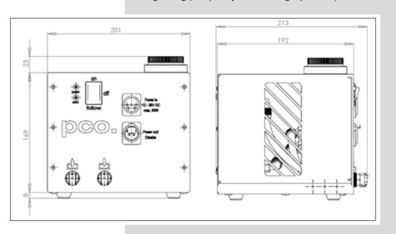
All dimensions are given in millimeter. Weight: 4kg (completely filled cooling liquid tank)
