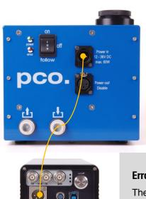
First connect the *Power out* of the cooling unit with the *Power* in of the pco.flim camera by using the PCO WAT camera cable. Or use separate power supplies for camera and aquamatic.
