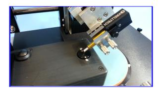
NOVA™'s Surface Videoscope allows the in-line inspection of polished surfaces while the component is still loaded in the polisher.
