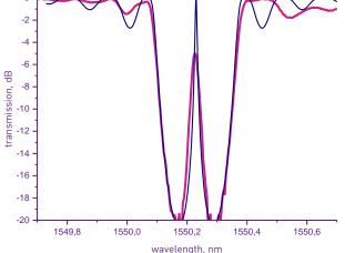
has a value 0.1nm ÷ 0.005 nm. Phase shifted FBGs are used as narrow bandwidth optical filter, for single – frequency fiber lasers creations. The experimental and theoretical transmission spectrum of FBGs is presented in the graph.
