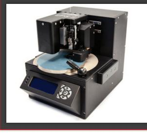
able performance and the bright, clear LCD screen guides the user with the correct action for each step. No special skill or "touch" is required –the EPS's precision fixturing holds the fibers precisely, and the automated system lowers the fibers smoothly onto the adjustable-speed polishing plate.
