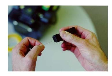
The FOSS-2001 Fiber Optic Smart Stripper employs precision design engineering and materials to gently remove the coating from 250µm fiber while placing near zero stress on the glass. The result — stress cracking and other similar damage to the fiber is virtually eliminated.
