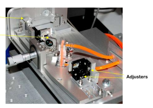
If the laser does not lase, try removing the tuning filter: it can be released by loosening the set screw in the top of the mount (0.7mm Allan key). Take great care not to touch the optical surfaces of the filter – wear finger cots.
