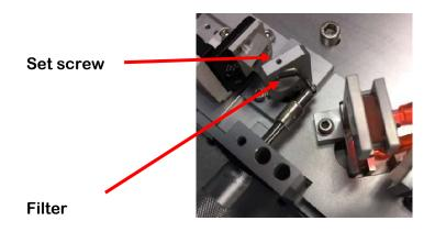
To change the filter, whilst wearing gloves or finger cots, loosen the set screw and carefully remove the filter, then replace with the other filter, and gently nip the set screw. DO NOT overtighten as this may crack the filter.
