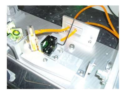
Monitor the laser power whilst making the adjustment to maximize the reading. This will approximate to best beam quality, but it is also possible to monitor beam quality on a suitable beam profiling system and adjust for the best beam.
