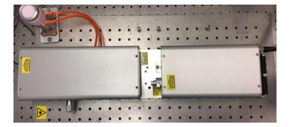
The position of the two heads, as factory tested, is marked by labels. Bolt down the SPOT and Dye laser heads to the plate using M6 bolts. (It will be necessary to take the lid off the dye laser to access the bolt holes). Align the edges of the heads to the edges of the plate. The heads could also be mounted directly to an optical table or breadboard with similar spacing.
