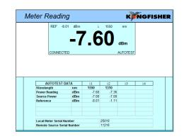
Live Data Sheet is for cable acceptance testing and instant pass / marginal / fail analysis at up to 4 wavelengths. Its main functions are on-site test configuration and acquisition. Project & instrument related information is also stored with the testing data. The sheet is auto-setup for 1 or 2 directional test during Autotest. In data Secure Mode, data is protected against unauthorized modification.
