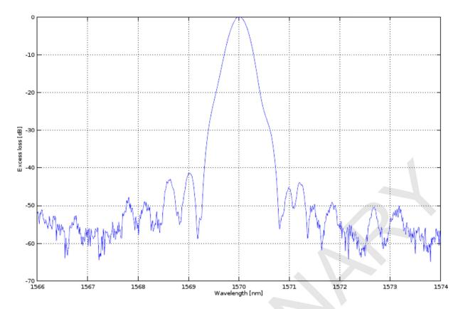
Figure 1 – Typical filter shape (model TFS1C509B)
