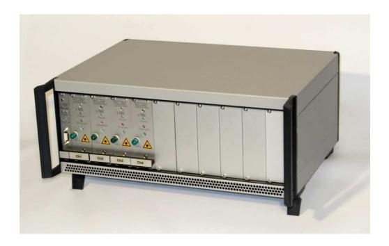
The LTBiS is a multi-channel laser diode drive system, that can be controlled through a digital electronic interface. The system design is modular, so that up to 10 laser diodes can be controlled independently within one 19''-instrument. Several instruments operated by one PC can be combined in a rack. A rack with the half width that fits with 4 plug-in units is available as an option.
