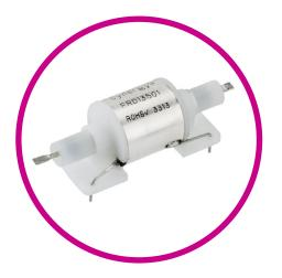
A complete RF screen around the coil assembly for a low loss transmission path, results in better carry current at elevated temperatures for this open frame series. An anti-corona sleeve is fitted around the reed switch for improved RF voltage isolation.
