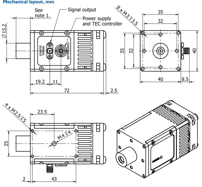
1. TO8 detector dimensions in the "TO8 technical drawing".
