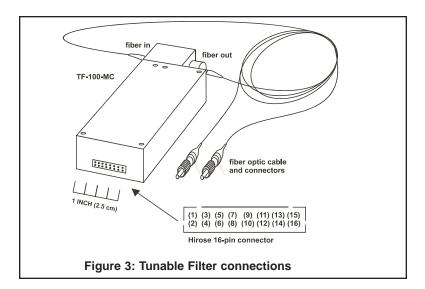
**Mounting:** The base of the TF-100-MC has three 2-56 tapped mounting holes for attachment to a rack or printed circuit board. For best results, the mounting surface should be rigid and free of vibration. Do not over-tighten the mounting screws and use screws with a threaded length no longer then 2mm.
