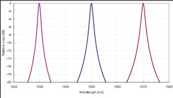
Figure 1: Typical Transmission Curves Of 1.2nm C-band **Tunable Filters**
