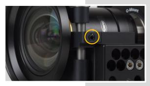
**Hexagon socket (Allen) set screw:** finally fix the screw on both sides of the lens cage with a tightning torque of 2.5 Nm.
