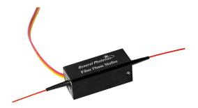
General Photonics' all fiber phase shifter/modulator provides phase shifts up to  $15\pi$  at frequencies from DC to 20 kHz. The all fiber construction practically eliminates insertion loss and back reflection. This compact device is ideal for fiber laser systems, fiber resonators, and fiber interferometers for precision phase tuning or phase modulation.
