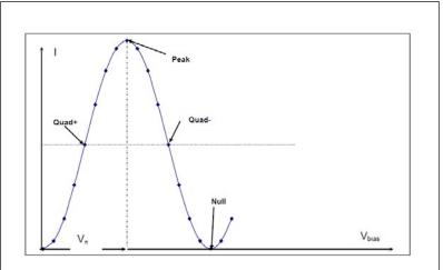
Figure 1. MZ modulator working function.
