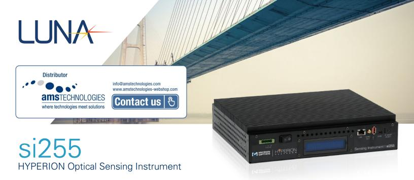
Luna's Micron Optics HYPERION si255 is an industrial grade fanless optical sensing interrogator. Featuring both static and dynamic full spectrum analysis, the si255 provides long-term, reliable and accurate measurements of nearly 1000 sensors on 16 parallel, 160 nm wide channels.
