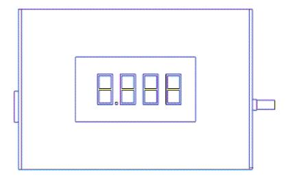
The display shows "X.XXX" which is in 'A', e.g. 0.025 means 0.025A which is 25mA.
