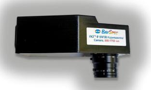
OCI-F-SWIR hyperspectral camera with a standard lens. The package is easy to mount on tripods or gimbals. Total weight ~820 g
