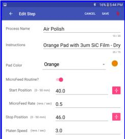
NOVA™ features an intuitive user interface for creating polishing programs. All parameters including cycle time, pressure and speed settings are easily inputted for all component types and desired surface geometries.
