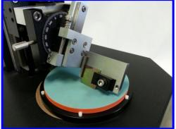
NOVA's versatility provides the ability to support the polishing of many photonic components. A quick change-out of workholder fixtures provides processing capability for waveguides, optical chips, PLCs, lenses and fiber arrays.
