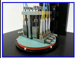
NOVA™ workholders feature patented independent KrellTech's suspension at each connector position for controlled pressure and uniform contact. Combined with NOVA's Microfeed™ fixture advancement, "airconnector polishing" and epoxy removal can be performed directly in the machine.
