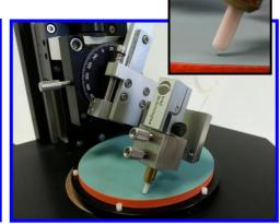
Bare fiber can be polished at variable angles using specialized workholders and adapters.=
