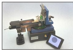
Krell's SpecVision<sup>™</sup> In-line Videoscope can engage with SpecPro<sup>™</sup> to inspect connector and fiber surface finishes while the component is loaded in the polisher.
