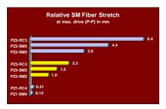
The **OPTIPHASE** PZ3 is the mid-range member of our family of fiber stretchers. It is a fiber wound piezoelectric element for use in a wide range of optical interferometric measurement and sensing system applications. Typical uses include open loop demodulation, sensor simulation, variable optical delay, general purpose fiber interferometry and large angle modulation of interferometric phase.
