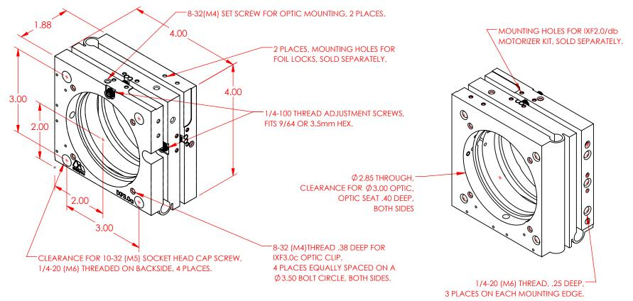
DIMENSIONS IN PARENTHESES REFLECT METRIC ASSEMBLY FEATURES
