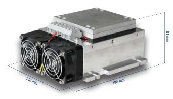
The compact thermoelectric plate-to-air cooling unit was developed for precise temperature control of laser diode modules and direct heat transfer to the ambient air. The highly efficient, solid state unit reaches a cooling capacity of 130 W for 24 VDC supply voltage and +25°C on laser mounting plate and +25°C ambient temperature.
