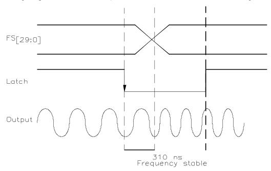
To generate a ferquency chirp, set the starting frequency as above and then apply the delta word to the FS input. A falling edge on DLATCH will then load the delta frequency word and initiate the chrip. The chirp will stop and output will return to to starting value or a rising edge.
